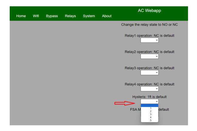
you change this setting until you find where the relay unwantedly is turning on / off to save the contacts of the LAC and the contactors / controls on the crane.
