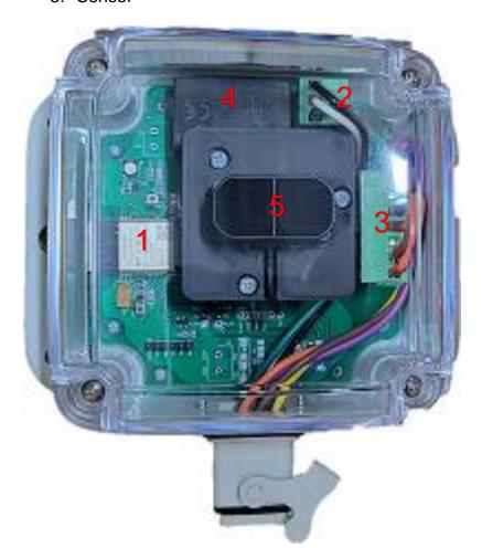
The LAC-12 has a 12 Meter (38ft) Range with 2 relay setpoints The relay setpoints are adjustable via the LAC-12 Webapp and real time distance is available in the webapp as well as the relay status of each relay.
