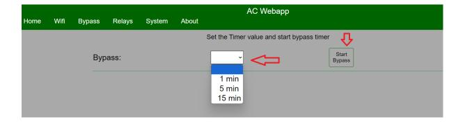
The Bypass button is not permeant due to safety reasons. You can choose 4 settings for bypass to help move the crane if it is stuck or if you haven't finished installing the system yet and need to move the crane.
