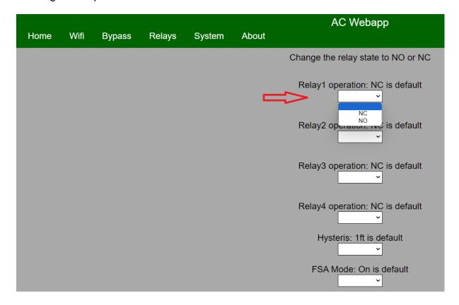
To Change the operation of the relay Pick the relay you want to swap the contact via the drop down menu and change it from NC to NO
